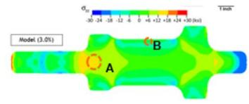
Qualifying RS at location A is inferred based on measured data at location B, and computed relationship between A and B Note that RS modeling is regarded critical to broad implementation of RS in design and structures assessments.
